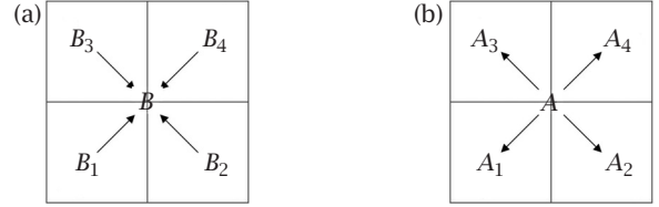
Figure 5 A basic observation that speeds up the computation of f_B and u_A . (a) f_B can be computed directly from f_{B_i} , where the B_i are B 's children. (b) Instead of adding u_A directly to all the points in A , we only add to u_{A_i} , where the A_i are A 's children.
