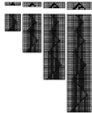
To emulate t steps in the evolution of the cellular automaton takes the Turing machine 2t^2 + 5t - 6 steps.
