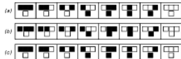
Sideways evolution in rule 30. (a) shows ordinary evolution from one row to the next. (b) shows evolution to the left starting from a pair of adjacent columns. (c) shows how a second column can be filled in from a row of cells to the right. The possibility of (b) is a consequence of one-sided additivity in rule 30; it leads to some level of cryptanalysis if the encrypting sequence consists of a complete column of cells.
