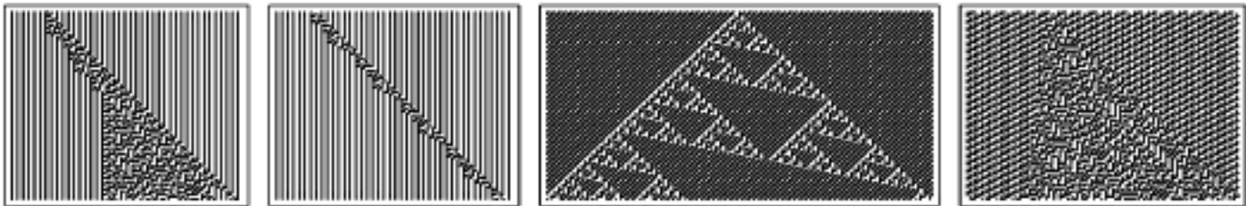
Examples of patterns produced by inserting a single extra black cell into repetitive backgrounds for rule 45. Note the appearance of a slanted version of the nested pattern from rule 90. In rule 45, localized structures turn out to be fairly common—but as in rule 30 they always seem to move at the same speed, and so presumably cannot interact to produce any kind of class 4 behavior.
